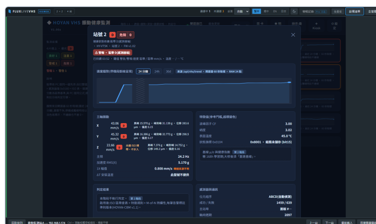
Device detail — triaxial vibration breakdown, feature values, trend and communication statistics, with the zone source and criteria version behind each verdict
