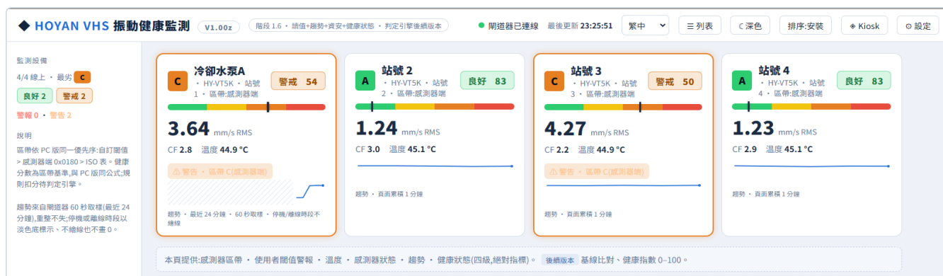
Light theme — two machines have fallen into zone C; the cards turn to the warning colour and show the alarm source. Screenshots are from a development build.
